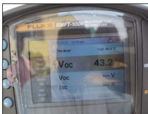
Fig.2: Measurement of Irradiation & Solar Cell Temperature ( T_{cell} ) without Non-woven fabrics Step 1: Estimation of Cell Temperature ( T_{cell} )
