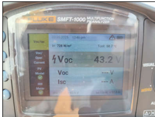
Fig 3: Measurement of Irradiation & Solar Cell Temperature ( T_{cell} ) with Non-woven fabrics Step 1: Estimation of Cell Temperature ( T_{cell} )
