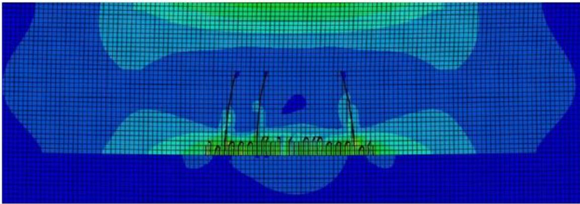
Fig. 3 Layer System and Crack propagation paths using FEM
