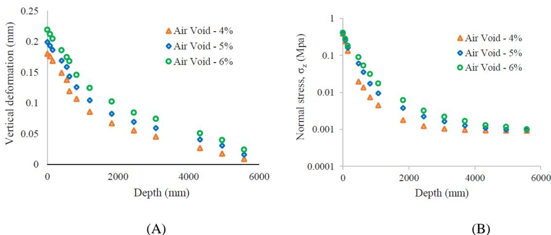
**Fig. 4.** (a) Pavement deformation vs. vertical depth (b) Normal compressive stress vs. pavement depth.
