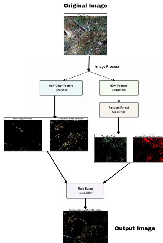
**Fig. 3** Integrated system architecture combining digital image processing and machine learning pipelines for comprehensive agricultural runoff detection.
