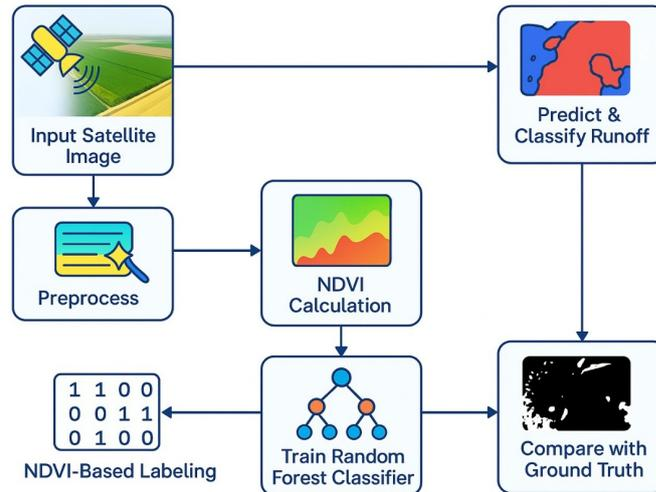
**Fig. 2** System Architecture for Machine Learning-Based Runoff Classification Framework
