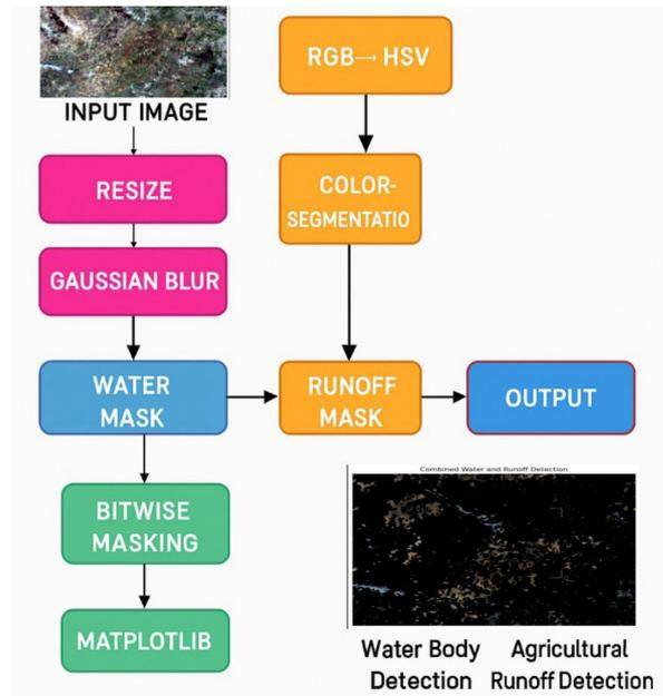
**Fig. 1** System Architecture for Digital Image Processing-Based Monitoring of Agricultural Runoff
