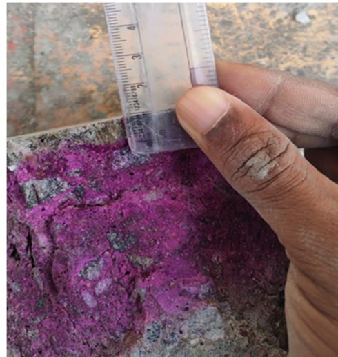
Fig: 4 Carbonation depth measurement
