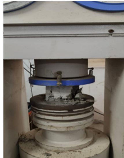
Fig:2 Failure pattern of specimen
