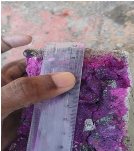
Fig .3 Carbonation depth measurement
