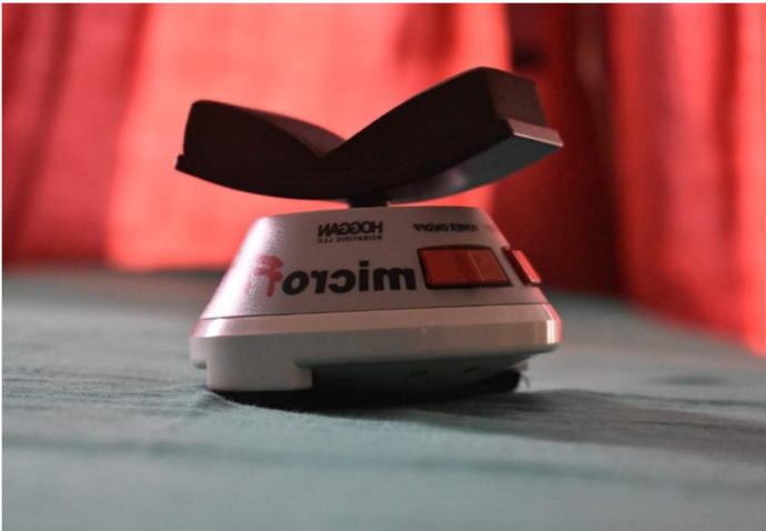
Figure-1 Wireless MicroFET®2 portable dynamometer
