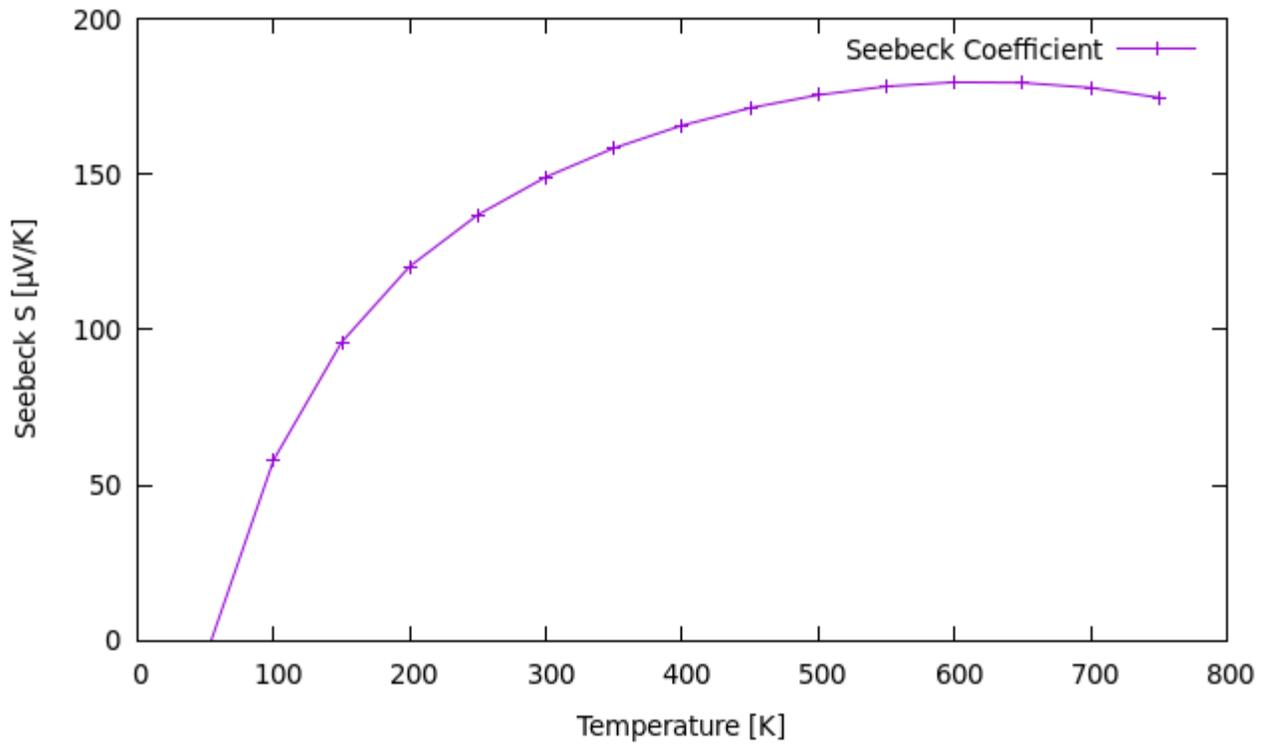
Figure 4. Seebeck coefficient with respect to temperature.
