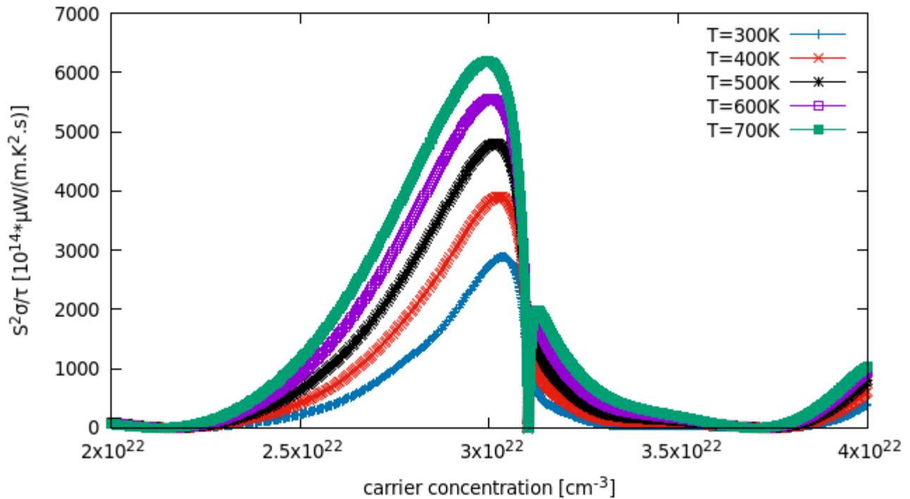
Figure 7. Power factor with respect to carrier concentration
