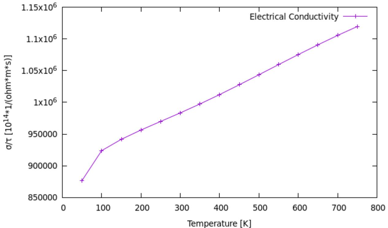
Figure 3. Electrical conductivity with respect to temperature.
