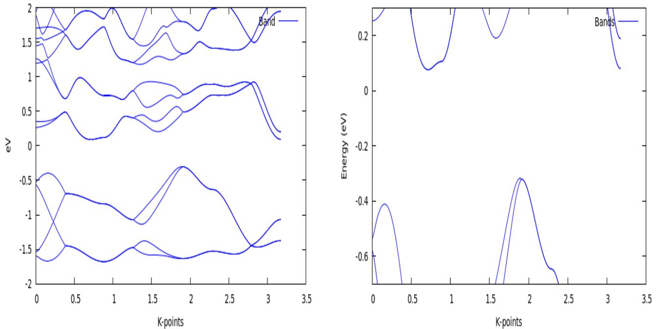
Figure 2, Electronic structure (Band Gap)  $E_g = 0.3962$  eV
