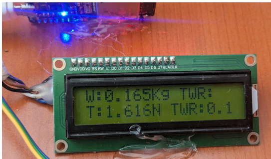
Figure 3.3. T/W/TWR values through LCD display Application
