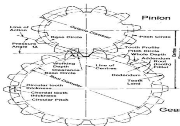
Fig No 5: Mating Spur Gear
